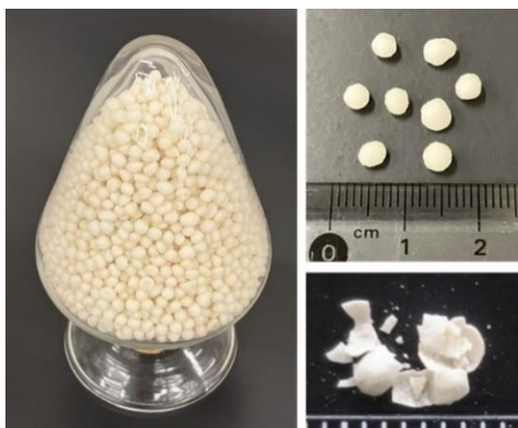
Photograph: Appearance of the Developed Product and the collapsed coated shell
